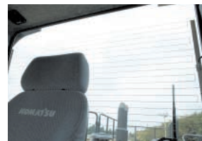
Rear heated glass provides clear view even in freezing or condensation conditions.
