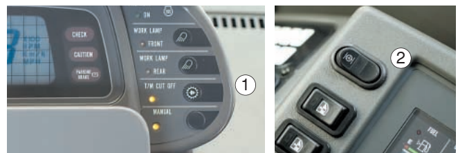
1:T/M cut-off ON/OFF switch 2:T/M cut-off set switch
