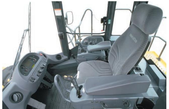
Noise at operator's ear noise level : 76 dB(A)
