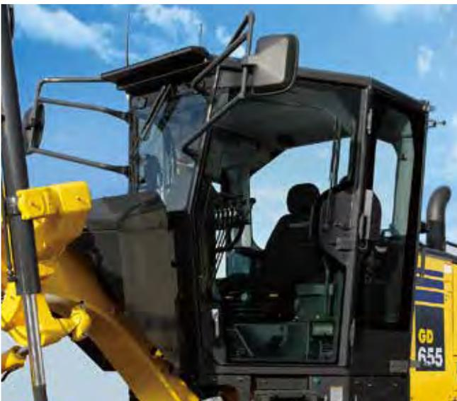
Low profile cab is designed to ensure ROPS/FOPS (ISO 3471/ISO 3449) certification.
