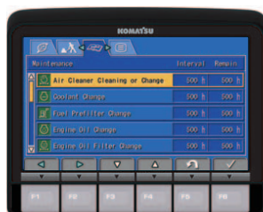
Maintenance List screen for replacement time display
