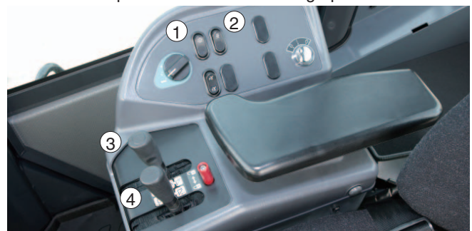
1:Cut-off ON/OFF switch 2:Cut off adjustment switch 3:Boom control 4:Bucket control
