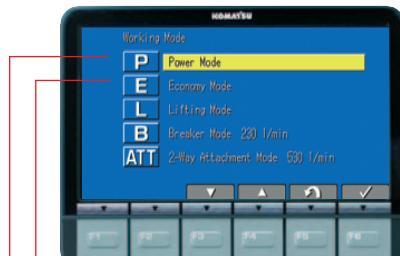
**E mode** – Economy or fuel priority mode further reduces fuel consumption, but maintains the P-mode-like working equipment speed for light duty work.
