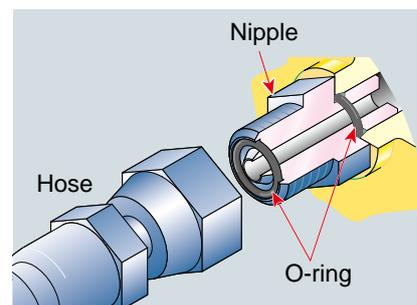
Flat face-to-face O-ring seals are used to securely seal all hydraulic hose connections and to prevent oil leakage.
