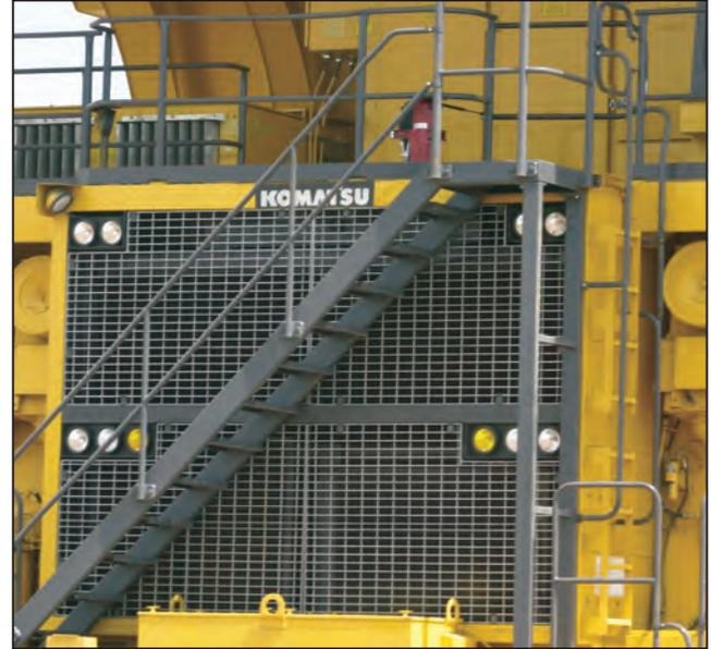
Komatsu's 960E-1 offers stairway access with entry from either the right or left side of the truck depending on the customer's preference.
